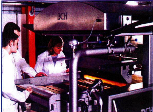
BCH Ultracoater enrobing wafer biscuits with caramel
